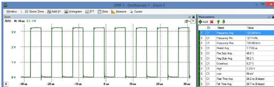
Figure 6-9: The GPIO C++ class flashing the LED
